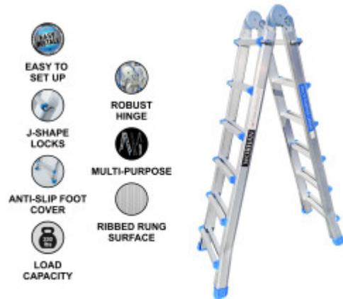
Ladder height (fully deployed): 18.4 ft. Ladder height (A-Frame at apex): 8 ft. 10 in. Number of rungs: 2 x 10. Rung spacing: 11.8 in. Product storage size: 64 in. x 17.4 in. x 9 in. Product weight: 32 lbs. Weight capacity: 330 lbs. Material: high-density grade aluminum.
